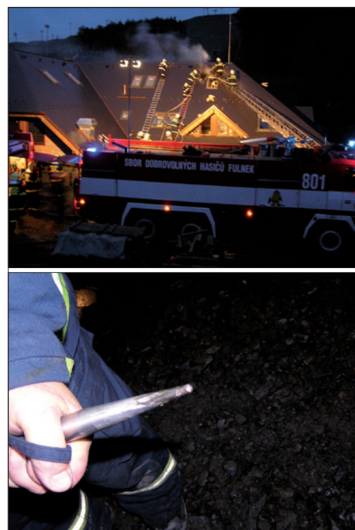
Fig. 1 Fire of the Odry hotel caused by lightning strike into ESE
